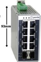
The IDS-710 is a 10 port Managed Ethernet Switch that can operate in industrial environments providing advanced performance and enabling real-time deterministic network operation. Eight 10/100/1000-Base-T Ethernet ports are available for networking Gigabit and Fast Ethernet devices. The two SFP slots support 10/100/1000 on Copper or 1G/2.5G on Fiber. This flexibility allows for easy adaptation to network growth and changes.
