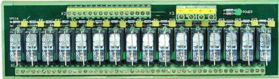
RM series power relay modules like RM-116 can be mounted on different DIN rail, such as TS-15, TS-32 or TS-35. Every channel of RM-104, RM-108, and RM-116 contains 1 Form C relay. The reverse polarity protection is provided to prevent improper operation. Every channel also has an LED to indicate its status. RM series modules include 4-channel relays, 8-channel relays and 16-channel relays versions for different applications.
